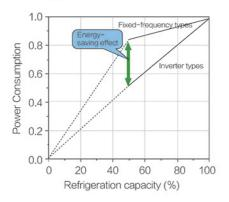
Vector frequency control is applied to reasonably distribute motor rotational torque to improve energy efficiency and save up to 38 % energy under some loaded conditions.
