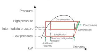
Under the working condition of high compression ratio, two-stage compression makes it possible to reduce power consumption, improve system COP, and obtain lower evaporating temperature.
