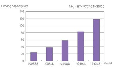
Note: Refrigeration capacity at the rotational speed of 2, 960 rpm and suction superheat of 5 °C, with an intercooler.
