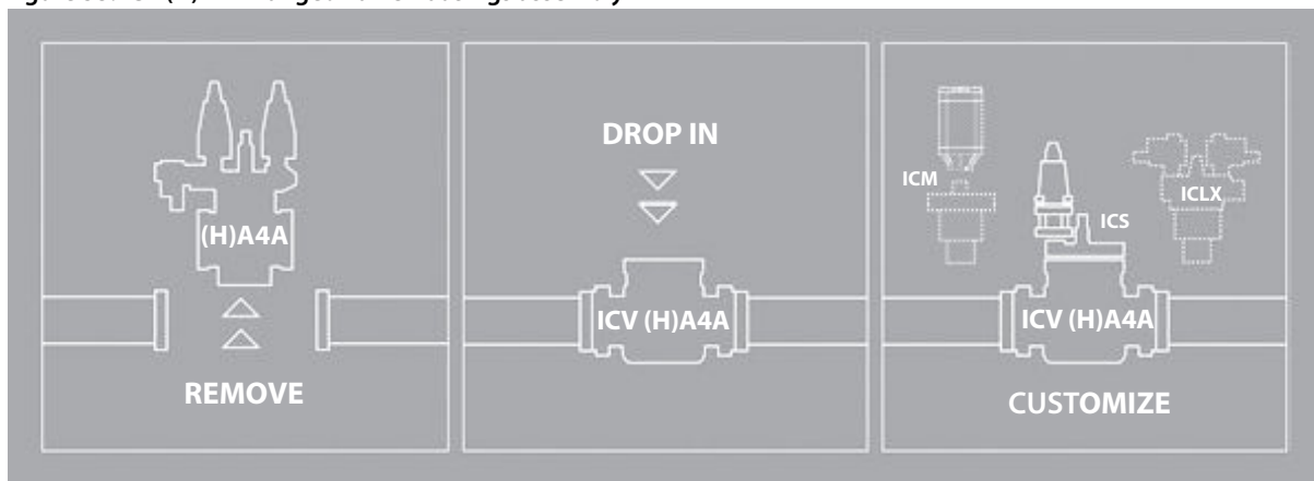
Figure 53: ICV (H)A4A flanged valve housings assembly
